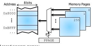
✓ A bank-switching scheme is preferred over a large linear address space. In systems with large linear address spaces, instructions require more bits for the address line, thereby increasing CPU overhead.
